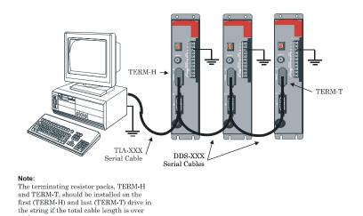
Figure 31: Multi-Drop Wiring Diagram
